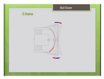
Like say for example, you can have a C frame connection like this, C frame connection between the tractor and the blade. So, with this particular kind of connection, certain types of movements of blade are possible. So, basically the connection between the tractor unit and the blade will decide what are the possible movements or the adjustments for the particular blade. So, we will discuss about the blade movements later.
