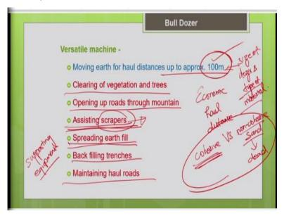
So, this bulldozer is basically a versatile machine. So, it can be used for different types of applications in a construction project site. So, before you select an earthmoving equipment for your particular activity or your particular job, you should know what is the haul distance actually
