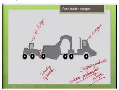
So, this is what I told you earlier, the bulldozer is used for assisting other machines, so it is supporting the other machines. So, this is your bulldozer, so this is a schematic sketch, so the leading one is your scraper. As I told you the scraper has to cut the earth and fill its bowl. So, during that loading operation, your bulldozer will push, you can see it has a special type of blade just for pushing it that blade is called as cushion blade.
