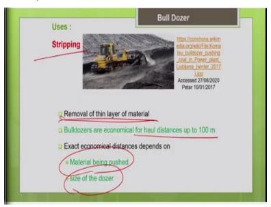
Then stripping, stripping is a very common operation in the construction project site. So, you know that stripping is nothing but removal of the top layer of the soil. So, if the top layer of the soil is weaker one with lot of vegetation, so you have to remove the top layer of the soil. So, depending upon a depth to which the vegetation is available in your soil accordingly you have to remove the top layer, so that is what is stripping.
