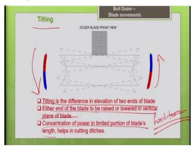
Now coming to tilting, tilting is the next type of movement. So, basically this is a movement in the vertical plane. So, you can raise one end of the blade and lower the other end. So, tilting is a difference in the elevation of the 2 ends of the blades; it is a movement in the vertical plane, why should we tilt the blade?
