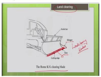
So, let us see some examples. Now you can see this bulldozer can be used for land clearing, so it is used for cutting the trees clearing your site. So, these are special bulldozers, for this purpose, we should not use a earthmoving blade, there are special land clearing blades. One such land clearing blade is Rome K bar G clearing blade, it is a very powerful blade, manufactured by Rome company.
