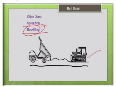
So, what are the other uses? The bulldozer can be used for spreading, backfilling. So, here you can see the example of spreading your truck. Very commonly you can see this in a road construction, the hauling equipment that is a truck, so it will dump the material and your bulldozer is used for uniformly spreading it and it will compact it to the regular thickness, so it helps in spreading the material.
