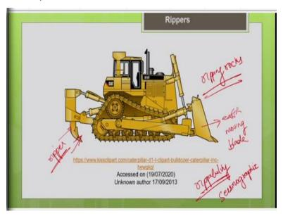
So, other application you can see it can be used as a ripper. So, for this tractor you can see a front end you have this blade earthmoving blade, this is the earthmoving blade, so at the rear end, you have this ripper. So, this is similar to plough what we use in farming. So, basically when we discuss about the earthmoving operations, the steps involved in the moving operations, I told you like the first step is we should loosen the earth before digging it.
