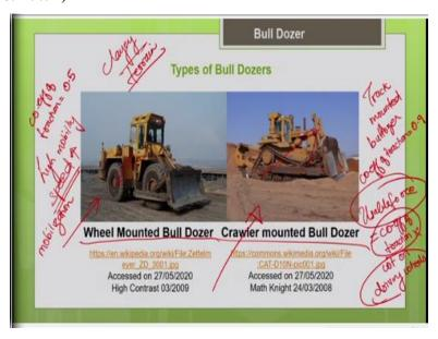
So, what happens if you go for say when you consider your track mounted or crawler mounted bulldozer. Here the coefficient of traction says it may be approximately 0.9 on a clayey terrain. So, here for the wheel mounted the coefficient of traction maybe only say 0.5. So, for the same weight of the machine since the coefficient of traction is very high obviously you can see with the usable
