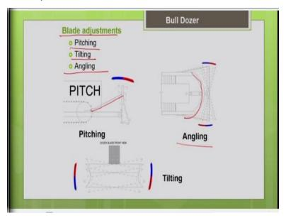
So, what are all the possible blade movements with the bulldozer blade? As I mentioned earlier, the movements which are possible depends upon the connection between the tractor and the bulldozer blade. In some bulldozers you can see this kind of C frame connection between the tractor and the blade. So, those tractors will facilitate certain kind of movements like angling.
