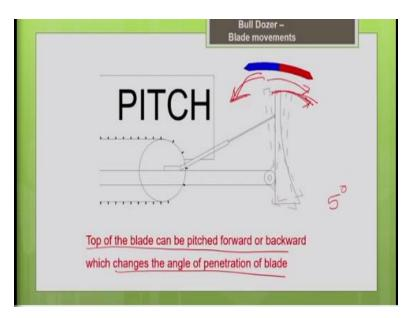
So, what is this pitching? Pitching means, the top of the blade is pitched forward or backward. That means you are moving the top end of the blade either forward or backward. So, this top end of the blade is moved forward or backward. So, why should we move it forward or backward? So, accordingly you can change your angle of cutting, accordingly you can change the depth of penetration of your blade.
